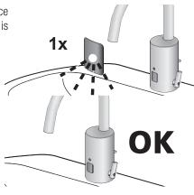
Press again (water flows) and release when the desired time of water flow (0-5 seconds) is reached.
